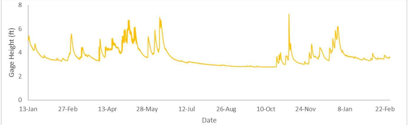
Note: Gauge height data was taken from USGS stream gauge number 14150290, 1.2 rkms downstream.
