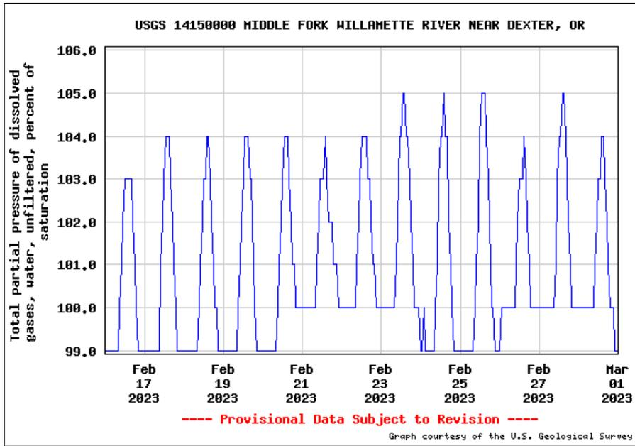
**Figure 44. Total Dissolved Gas Saturation (%); Middle Fork Willamette River, Near Dexter, OR**
