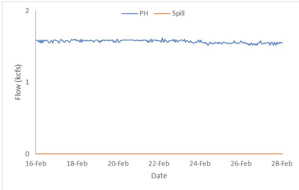
**Figure 46. Hourly Flows PWR vs. Spill (Dexter Dam)**
