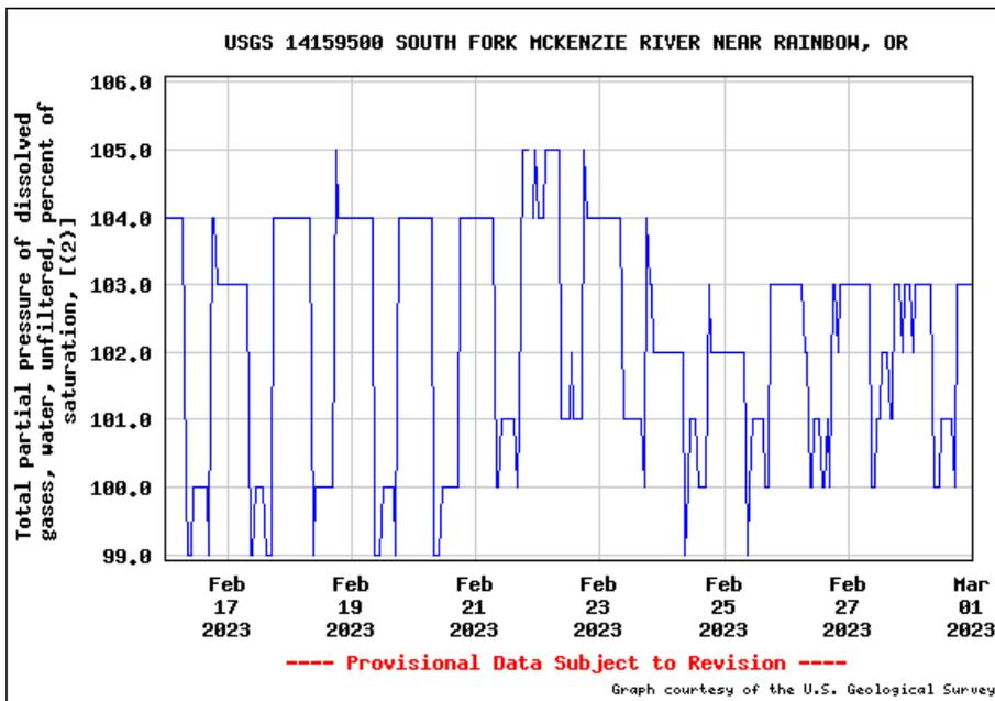
Figure 24. Total Dissolved Gas Saturation (%); below Cougar Dam, South Fork McKenzie River
