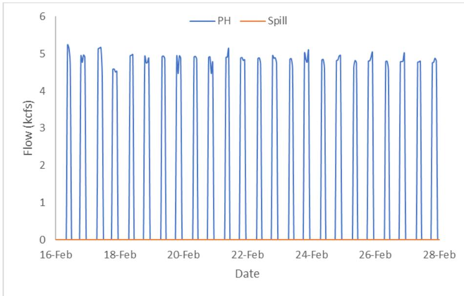
**Figure 52. Hourly Flows PWR vs. Spill (Lookout Dam Tailrace)**
