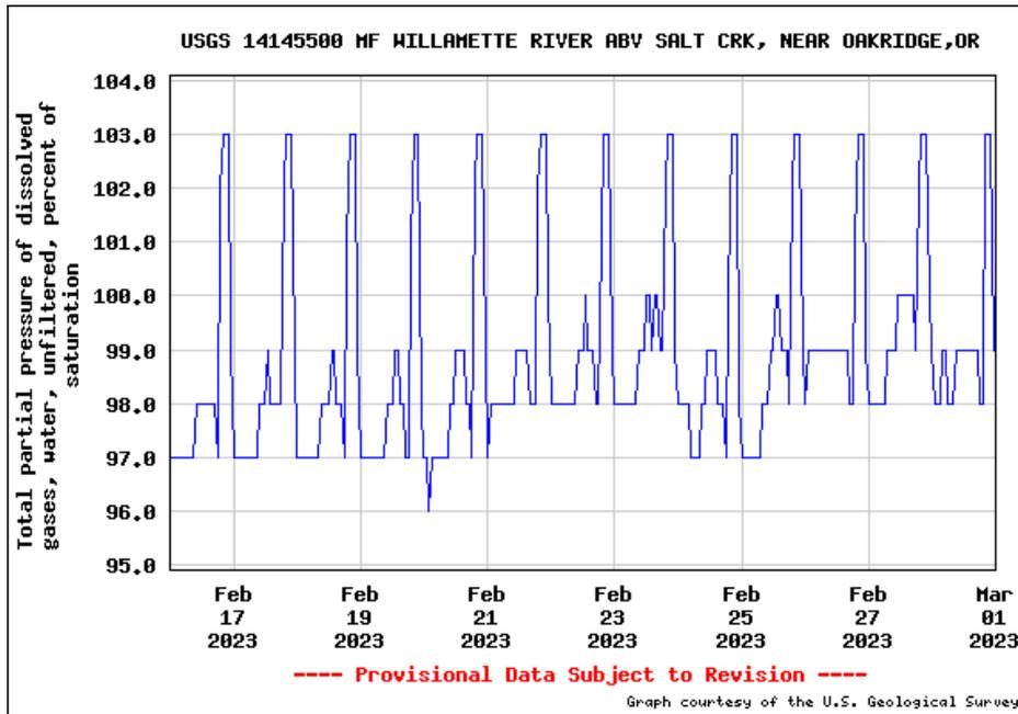
Figure 61. Total Dissolved Gas Saturation (%); below Hills Creek Dam – Middle Fork Willamette River
