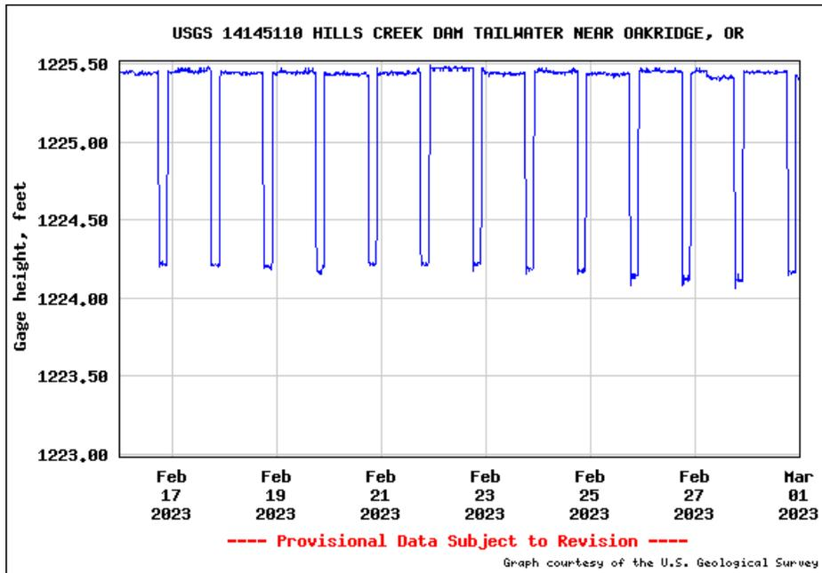
Figure 60. Gauge Height (feet); below Hills Creek Dam PWR - Middle Fork Willamette River
